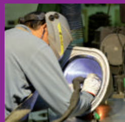
Welding stainless steel sanitary fittings DELABIE's factory in Aveiro, Portugal
