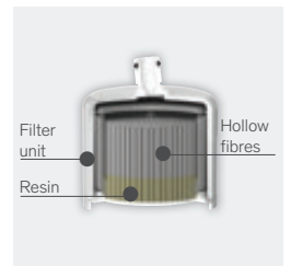
Section of the BIOFIL tap filter
