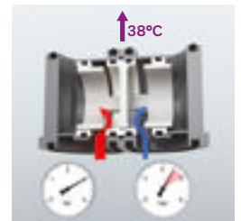
At 38°C: HW 3 bar/CW 2.5 bar
