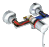
Smooth interior = very little biofilm Thermal insulation on HW side No non-return valves
