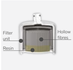
Section of the BIOFIL tap filter
