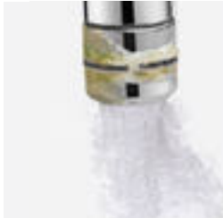
Scale build-up on aerator causes splashing
